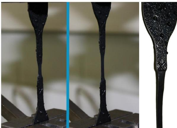
Naturally, the effect of a reduced elongation is more apparent in materials of high density which have a greater crystallinity and less for thinner materials with a lower crystallinity, such as linear or low density polyethylene.
