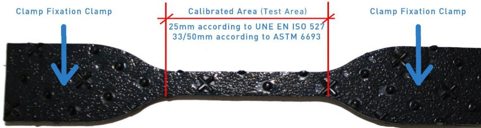
It is evident that the "texturing bumps" which are within the calibrated zone are basically a thickening of the membrane which will not deform in the same way as the rest, they are hard areas of between 2 and 4 mm in length which will not deform (see photograph).
