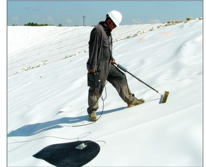
**Leak Detection Liner**
